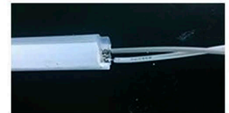
1. Cut at proper way to show the soldering place
